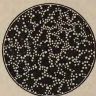
FIG. 15.—Appearance preceding coagulation in a concentrated gold solution. (According to H. Siedentopf.)
